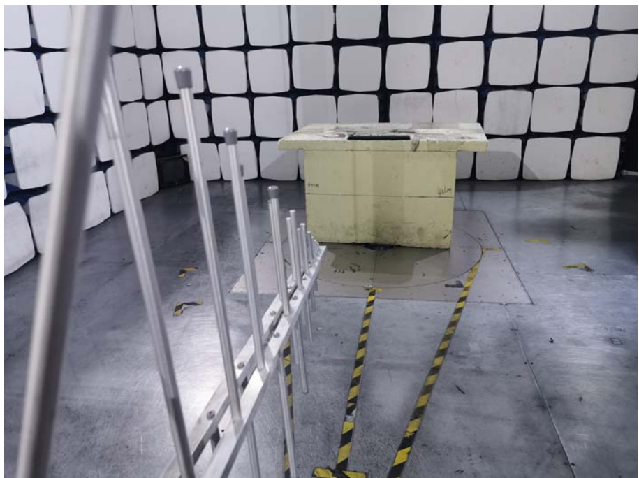
Radiation Emission Test Setup (30MHz to 1GHz)
