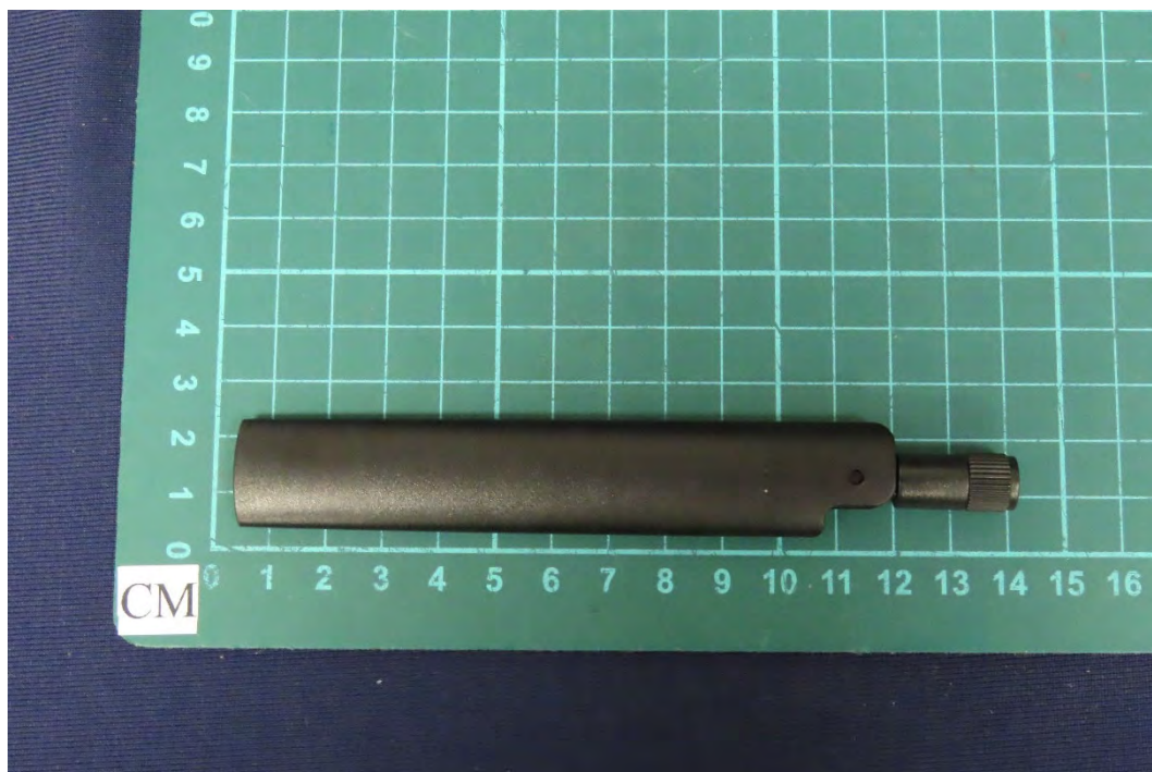
(33) EUT Photo GPS Antenna
