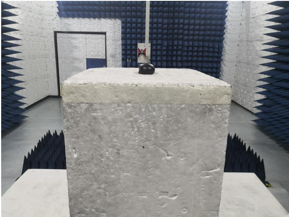
RADIATED EMISSION TEST SETUP ABOVE 1GHz
