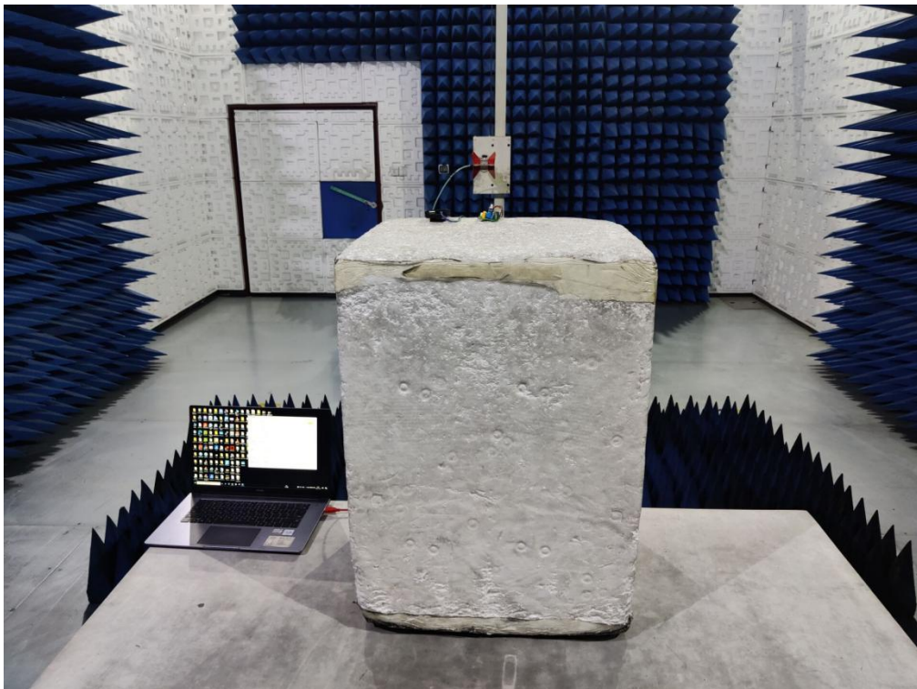
RADIATED EMISSION TEST SETUP ABOVE 1GHZ
