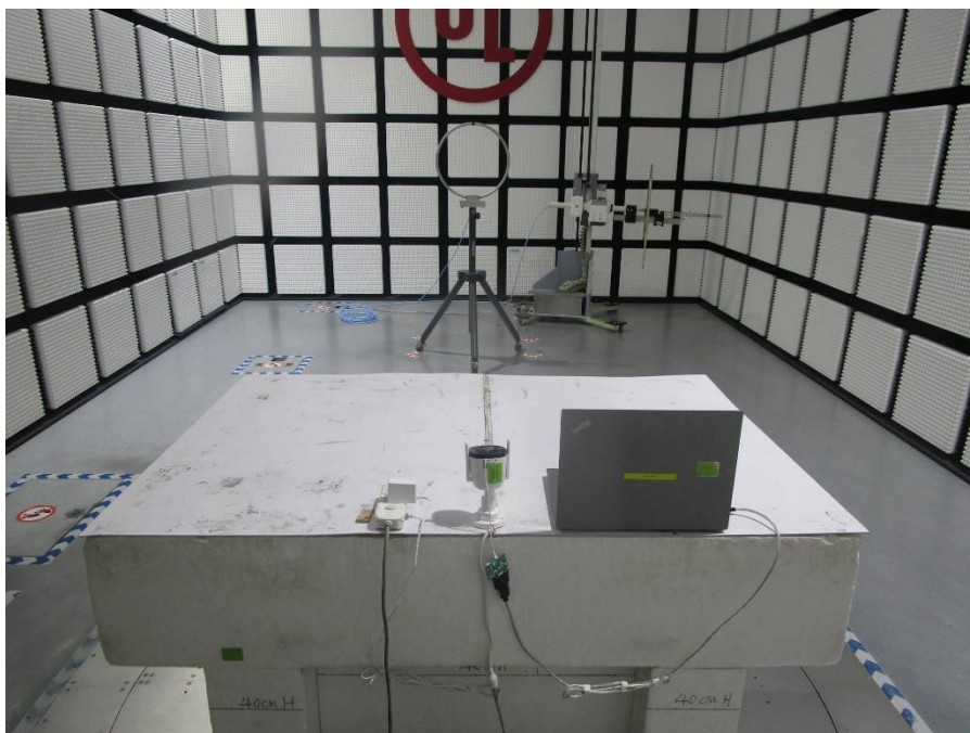
RADIATED RF MEASUREMENT SETUP (Below 30MHz)
