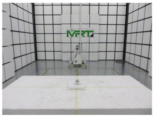
Description: Radiated Spurious Emissions Test Setup for Above 1GHz
