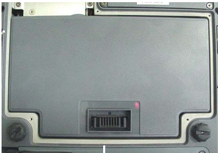
Internal Li-ion Battery 11.1 V, 3600 mAh (Model: T8M-E)
