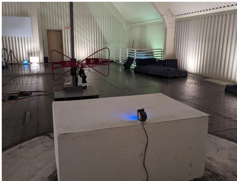
Photograph 2: Back View Radiated Emissions Worst-Case Configuration – Frequencies Below 1000 MHz
