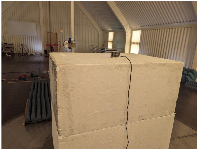
Photograph 4: Back View Radiated Emissions Worst-Case Configuration “Long Edge” Orientation – Frequencies Above 1000 MHz
