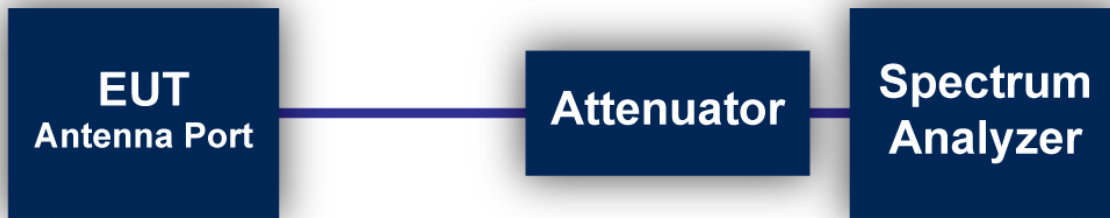
Figure 2: Direct Connection at the Antenna Port Test
