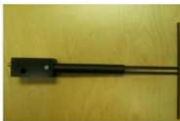
Figure 1 – MVG COMOSAR Validation Dipole
