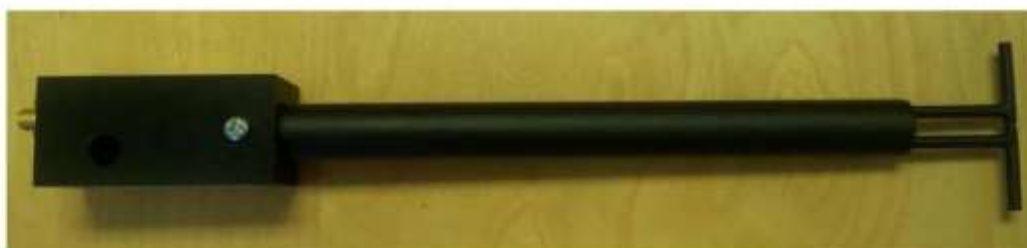
Figure 1 – MVG COMOSAR Validation Dipole
