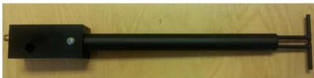
Figure 1 – MVG COMOSAR Validation Dipole
