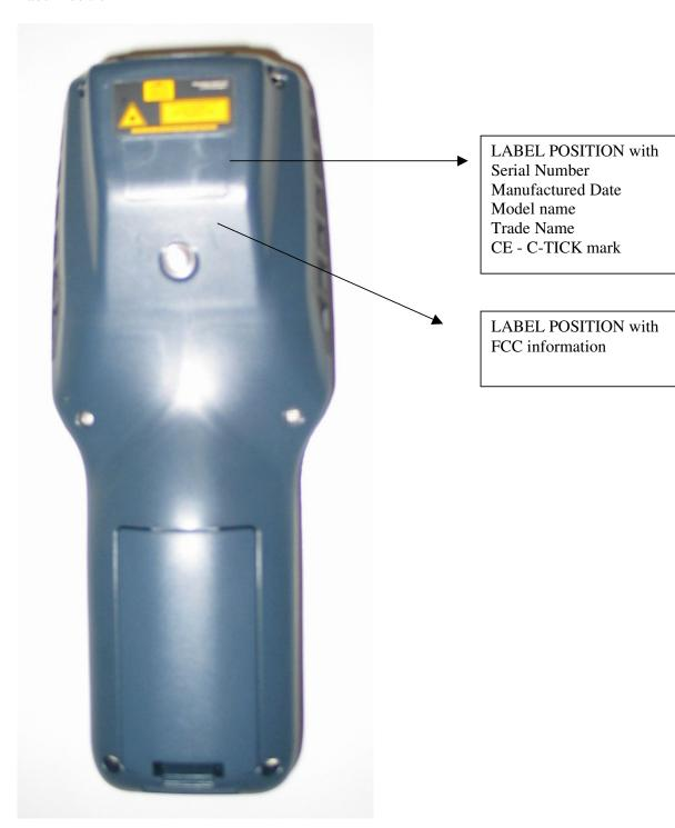
Label used in KYMAN-NET models with WI-FI, BT and GSM/GPRS
