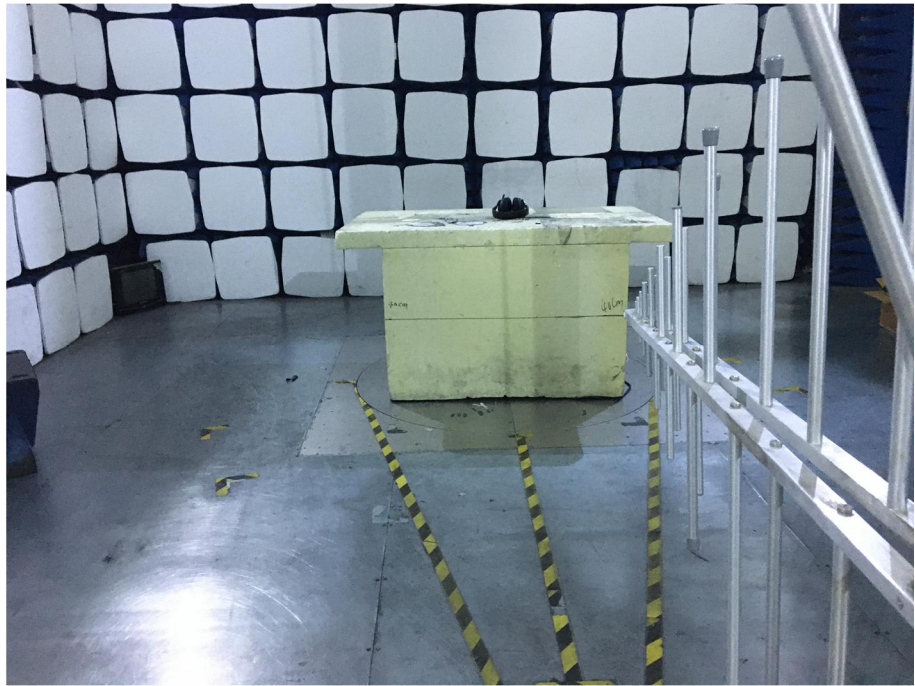
Radiation Emission Test Setup (30MHz to 1GHz)
