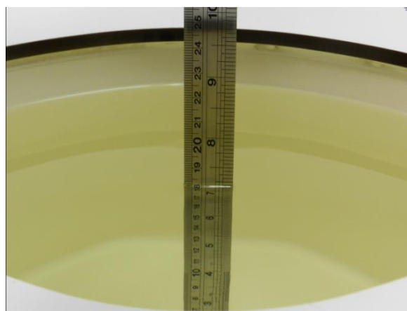
Fig 11.2 Photo of Liquid Height for Body SAR
