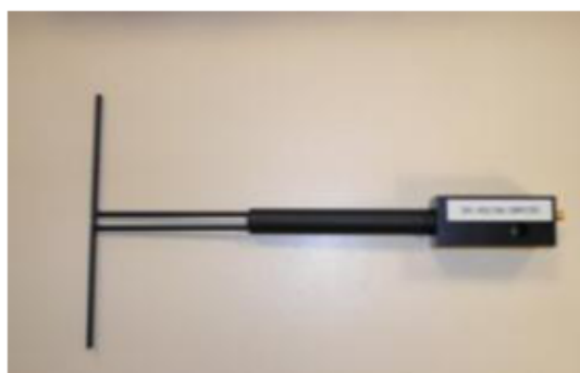
Figure 1 – Satimo COMOSAR Validation Dipole
