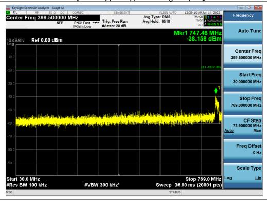
Antenna 1 / Low Edge - 100 MHz ~ Low Edge / (B5 DSS 10 MHz 1 Carrier + LTE B5 5 MHz 1 Carrier) + 5G NR n5 5 MHz 1 Carrier [3 Carrier] (2C+1C) / Non-Contiguous / 64QAM
