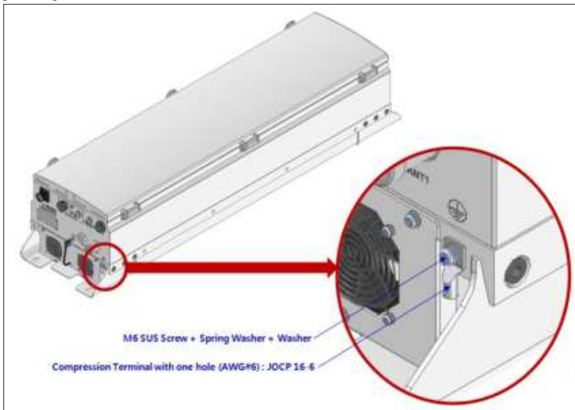
Figure 18. Location of Ground Terminal
