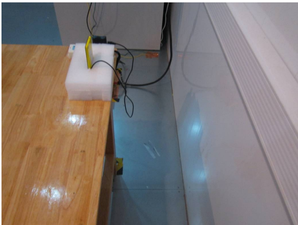
Conducted Emissions Test Setup Side View
