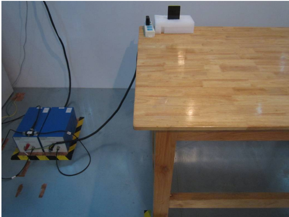
Conducted Emissions Test Setup Front View
