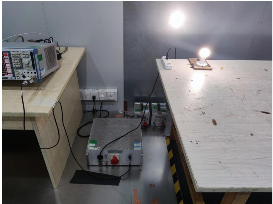
Conducted Emission Test Setup
