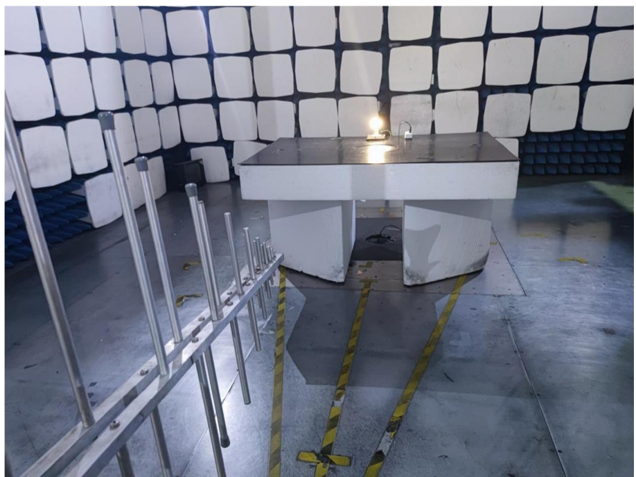
Radiation Emission Test Setup (30MHz to 1GHz)
