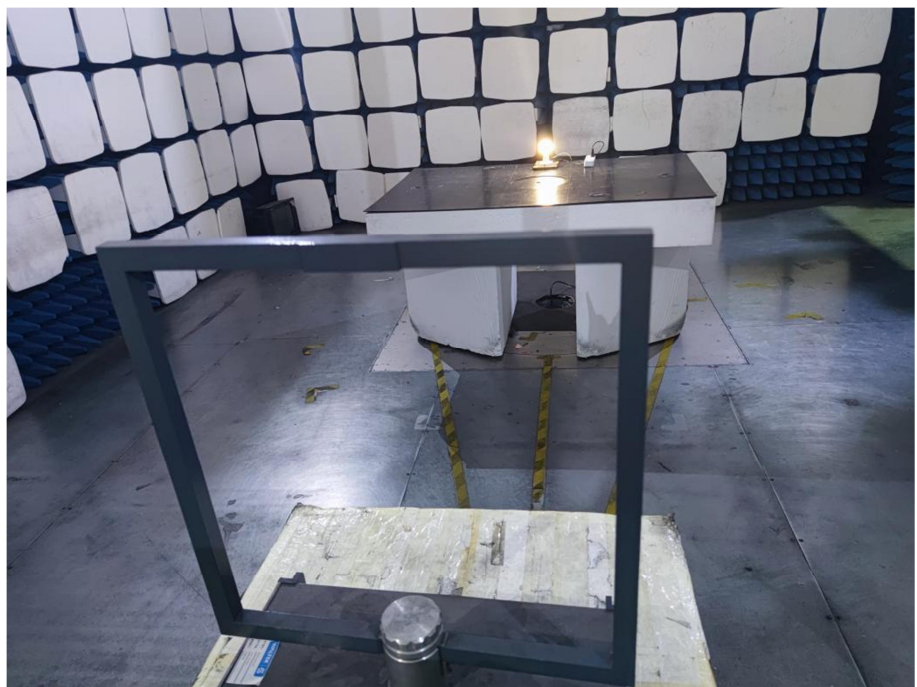
Radiation Emission Test Setup (Below 30MHz)
