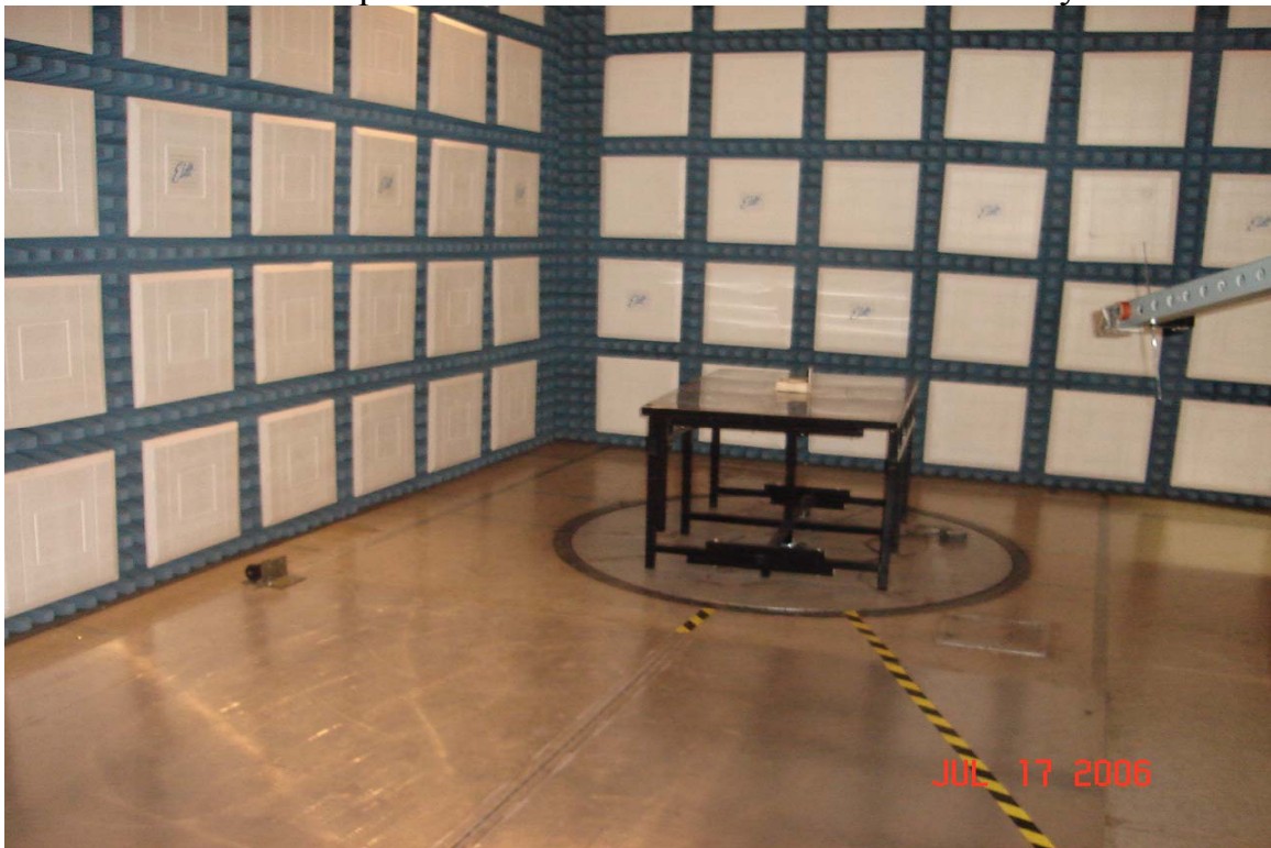
Test Set-up for Radiated Emissions Vertical Polarity
