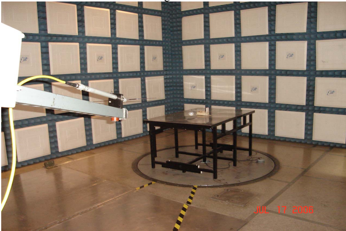
Test Set-up for Radiated Emissions Horizontal Polarity
