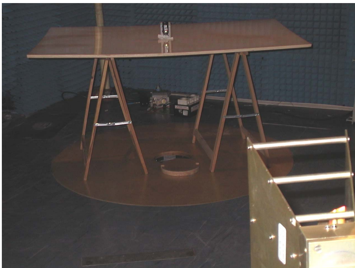
Photograph-4 Set up for Radiated Emission 1GHz-5GHz
