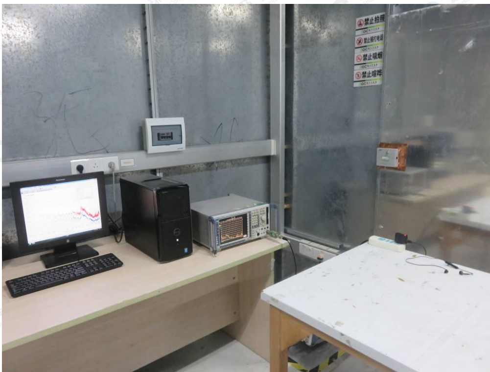
FCC RADIATED EMISSION TEST SETUP
