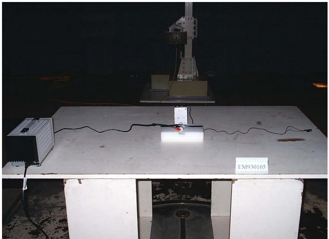
BACK VIEW OF RADIATED MEASUREMENT
