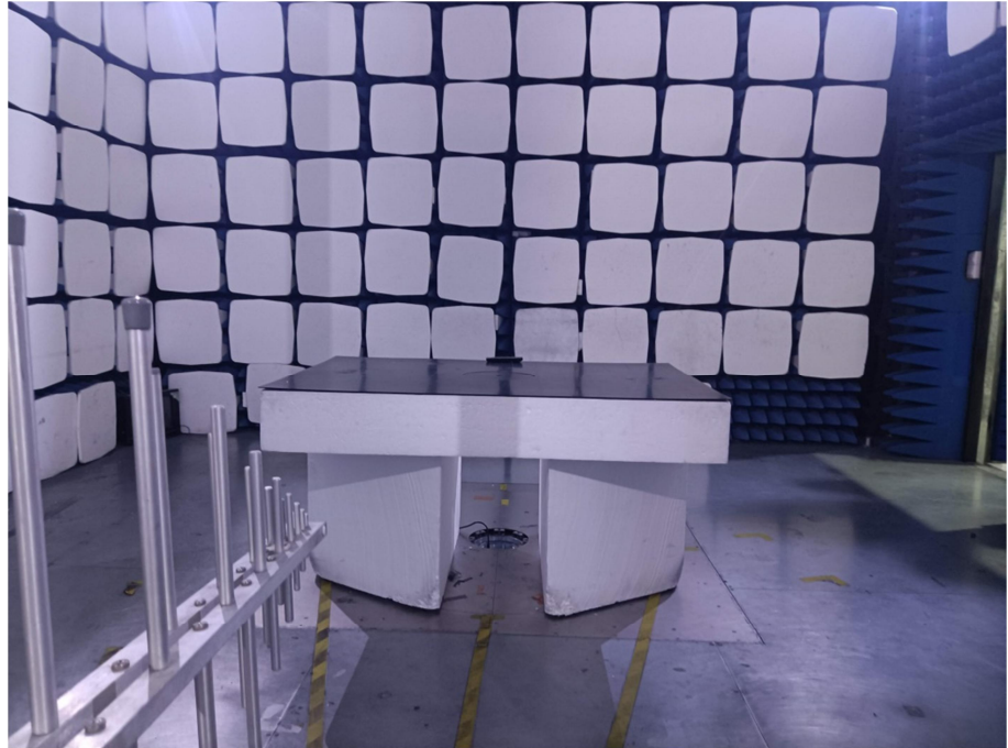
Radiation Emission Test View (30MHz to 1GHz)
