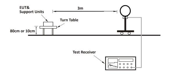
For Radiated emission 30MHz to 1GHz:
