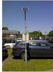
The Data Collector GPRS will not consume more than 60mA at 12VDC on average.
