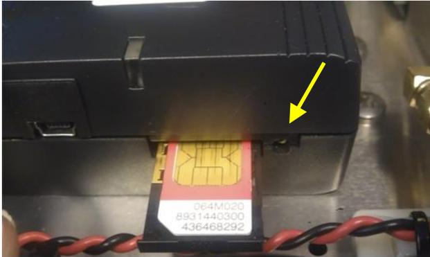
Figure 23: SIM Card installation
