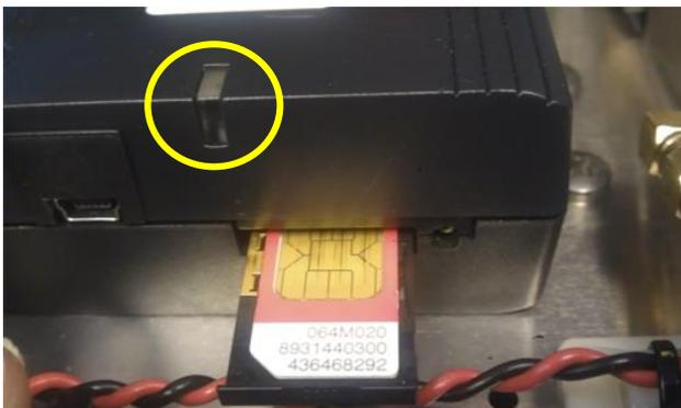
Figure 25: GPRS Modem status LED
