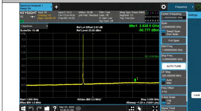
Band2-5MHz-QPSK-18625-1RB#24-1000~3000-PASS
