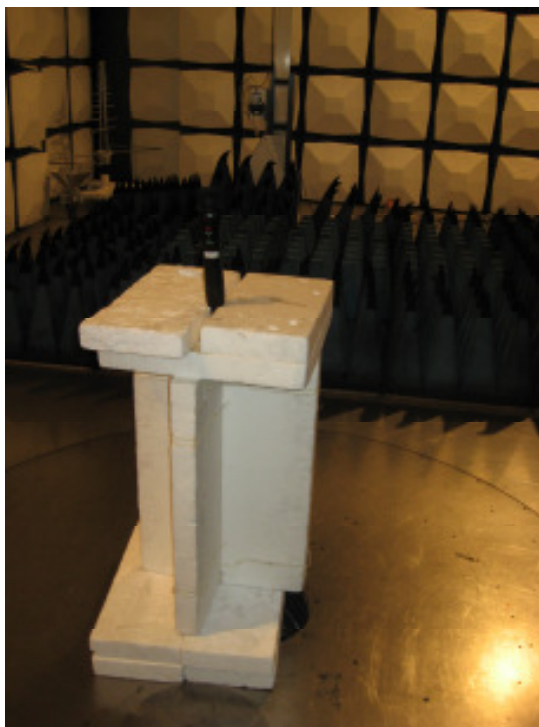
Photograph 2: Set-up for Radiation Measurement above 1GHz
