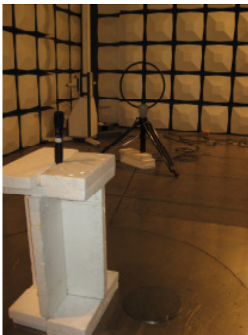
Photograph 1: Set-up for Radiation Measurement below 1GHz
