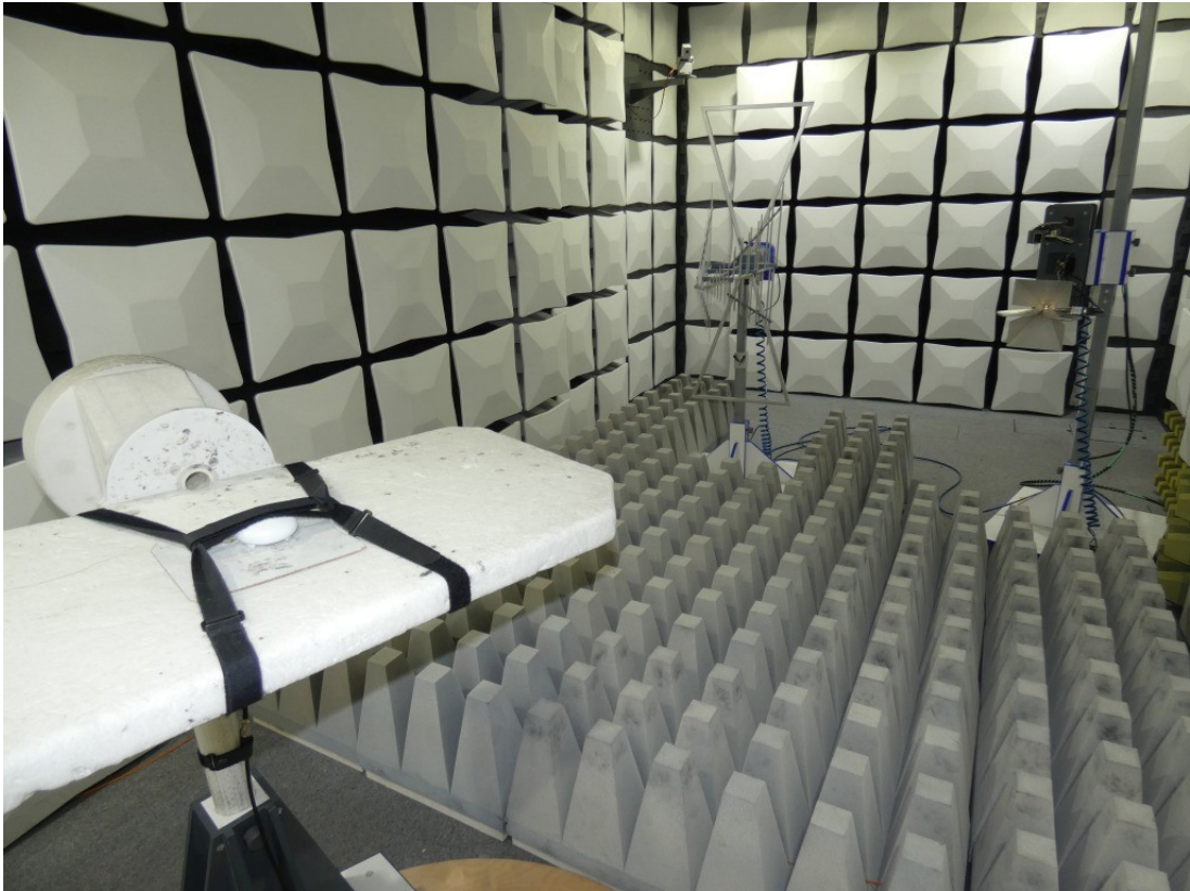
Photo 3: Test setup for radiated measurements above 1 GHz
