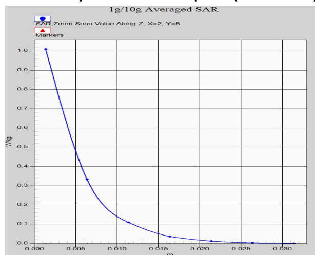
Z-Scan at power reference point (N78 ANT11)
