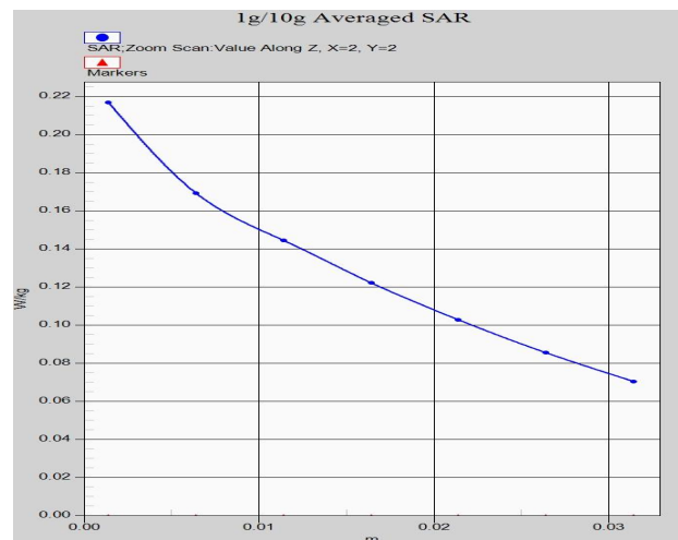
Z-Scan at power reference point (N5 ANT41)
