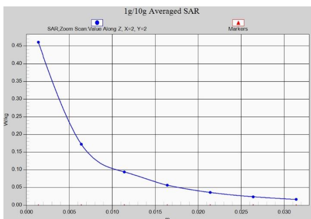
Z-Scan at power reference point (N5 ANT13)
