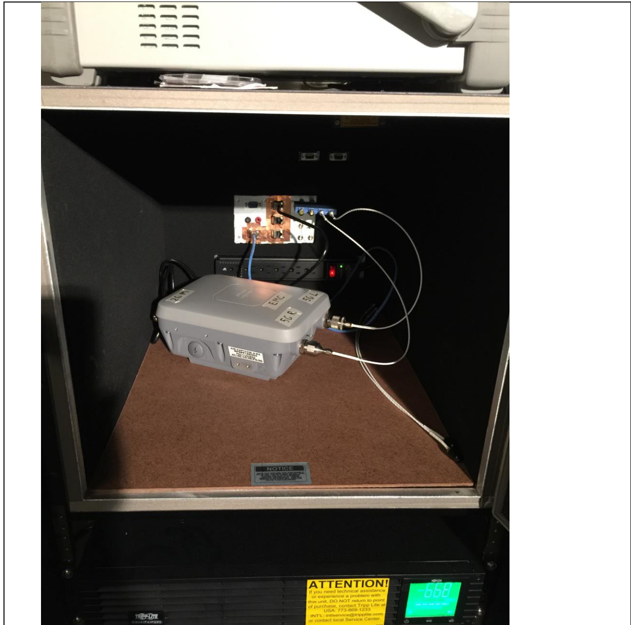
Title: AIR-CAP1532E-B-K9 Conducted Test Setup
