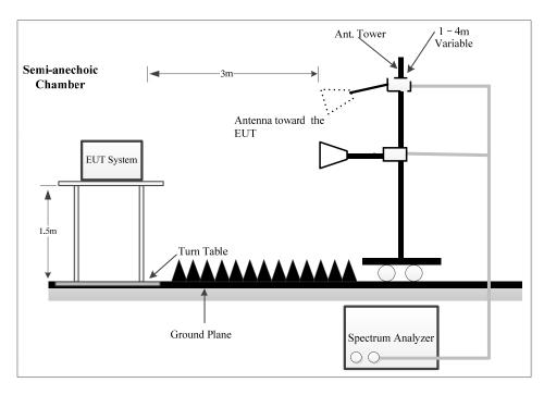
The radiated emissions were performed in the 3 meters distance, using the setup accordance with the ANSI C63.10-2013. The specification used was the FCC 15.209, and FCC 15.247,RSS-247,RSS-Gen limits.
