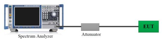
A short RF cable with low cable loss connected to the EUT antenna port, which was provided by manufacturer. The insert loss of this RF cable/attenuator was offset into the setting of test equipment.
