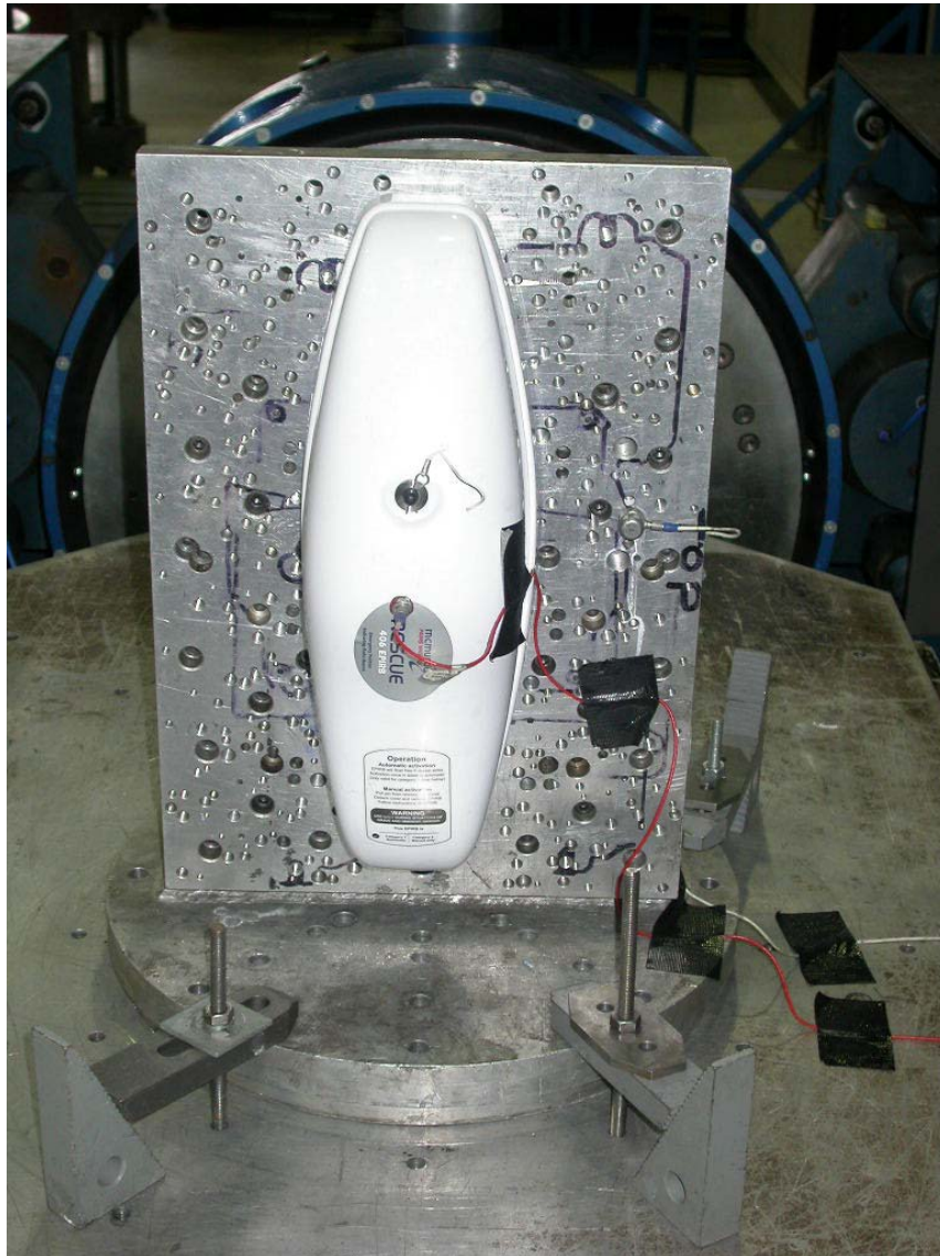
Photograph showing Vibration Test Set-up in Float Free Enclosure
