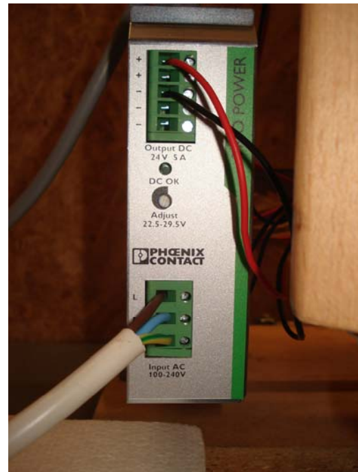
Photograph 2.3-2: Power supply TRIO-PS/1AC/24DC/5, front view
