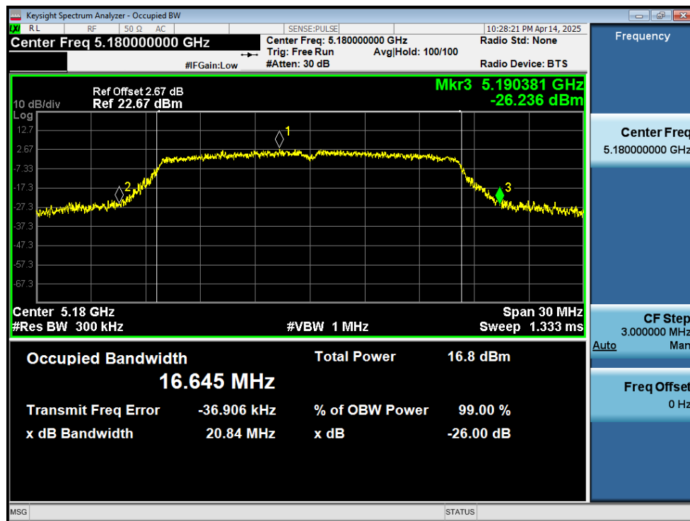
-26dB Bandwidth NVNT a 5180MHz Ant2
