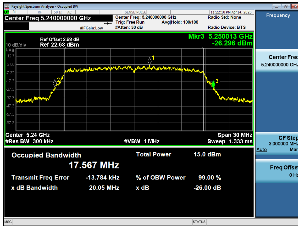
-26dB Bandwidth NVNT n20 5240MHz Ant1
