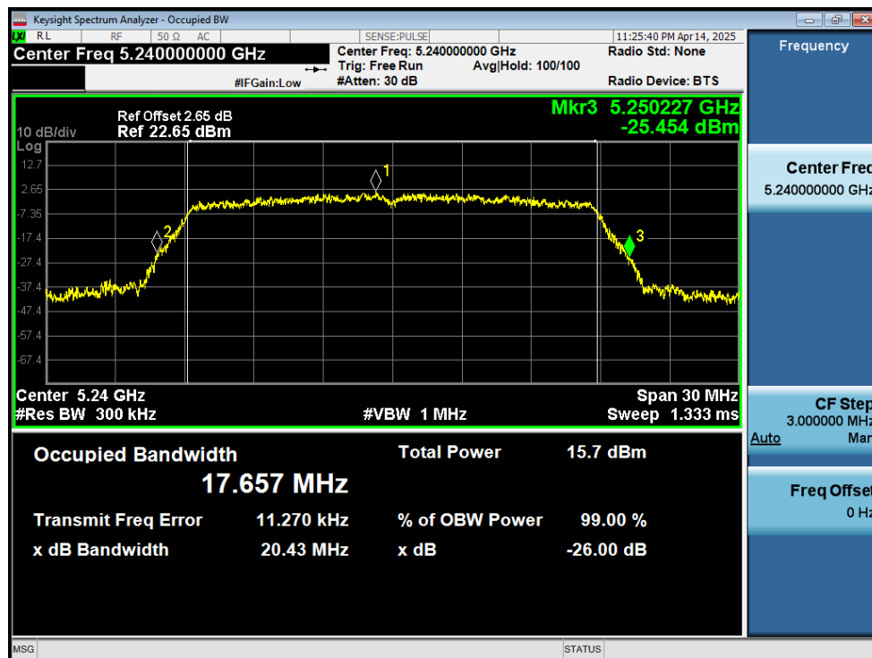
-26dB Bandwidth NVNT n20 5240MHz Ant2
