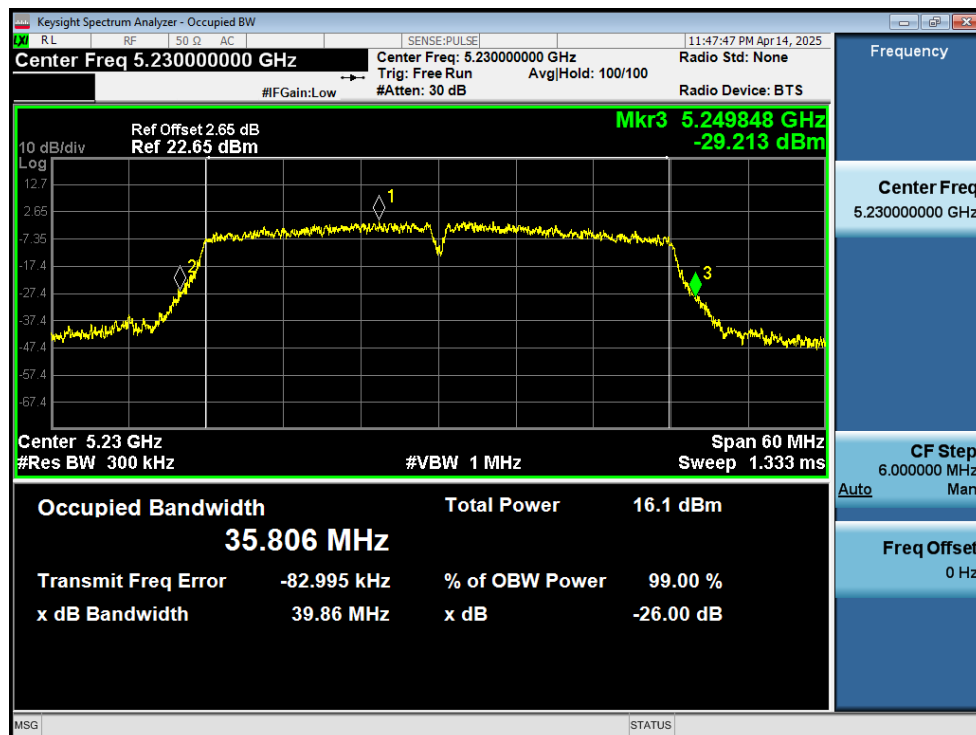
-26dB Bandwidth NVNT ac40 5230MHz Ant2
