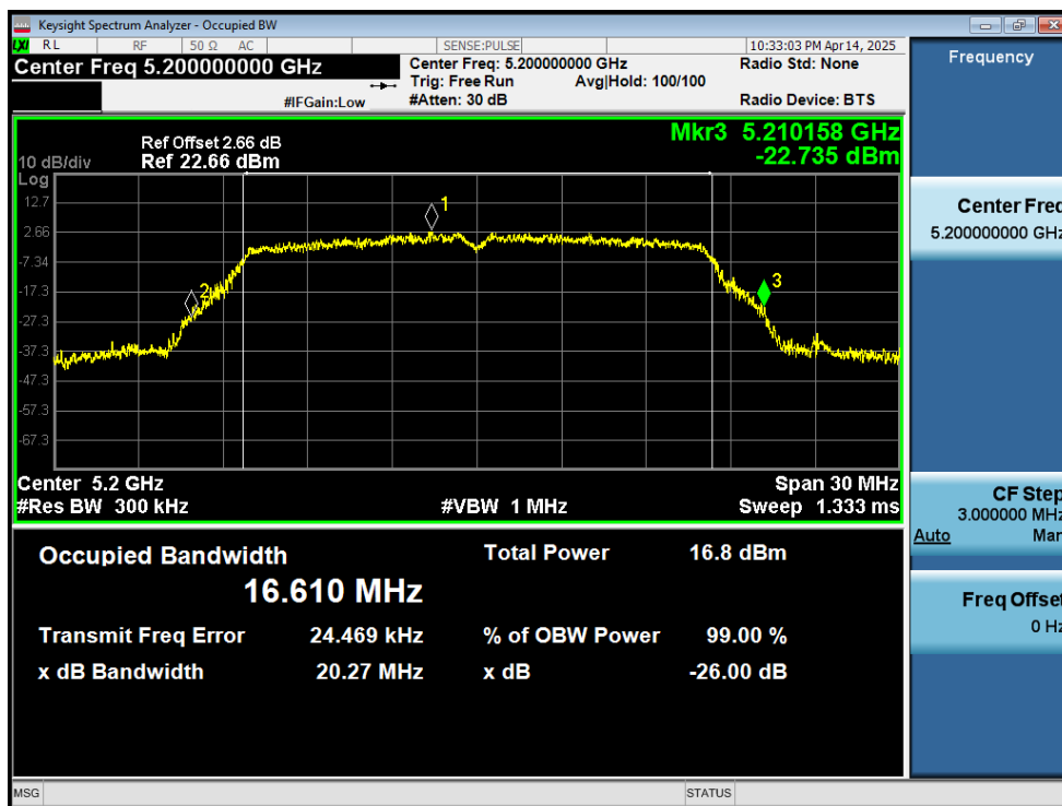
-26dB Bandwidth NVNT a 5200MHz Ant2
