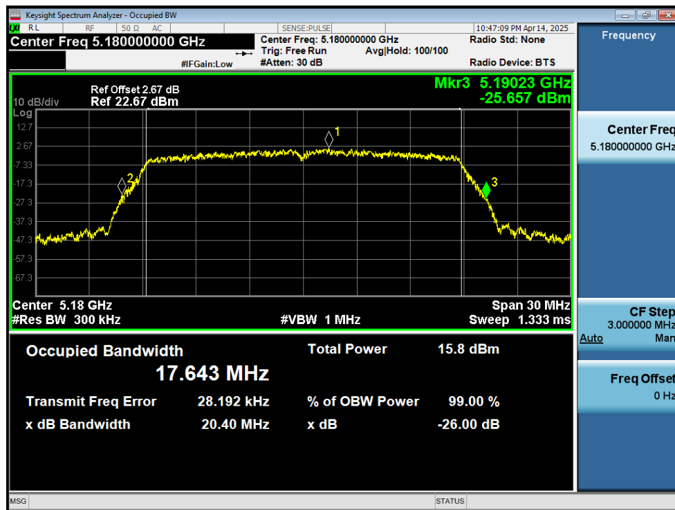
-26dB Bandwidth NVNT ac20 5180MHz Ant2
