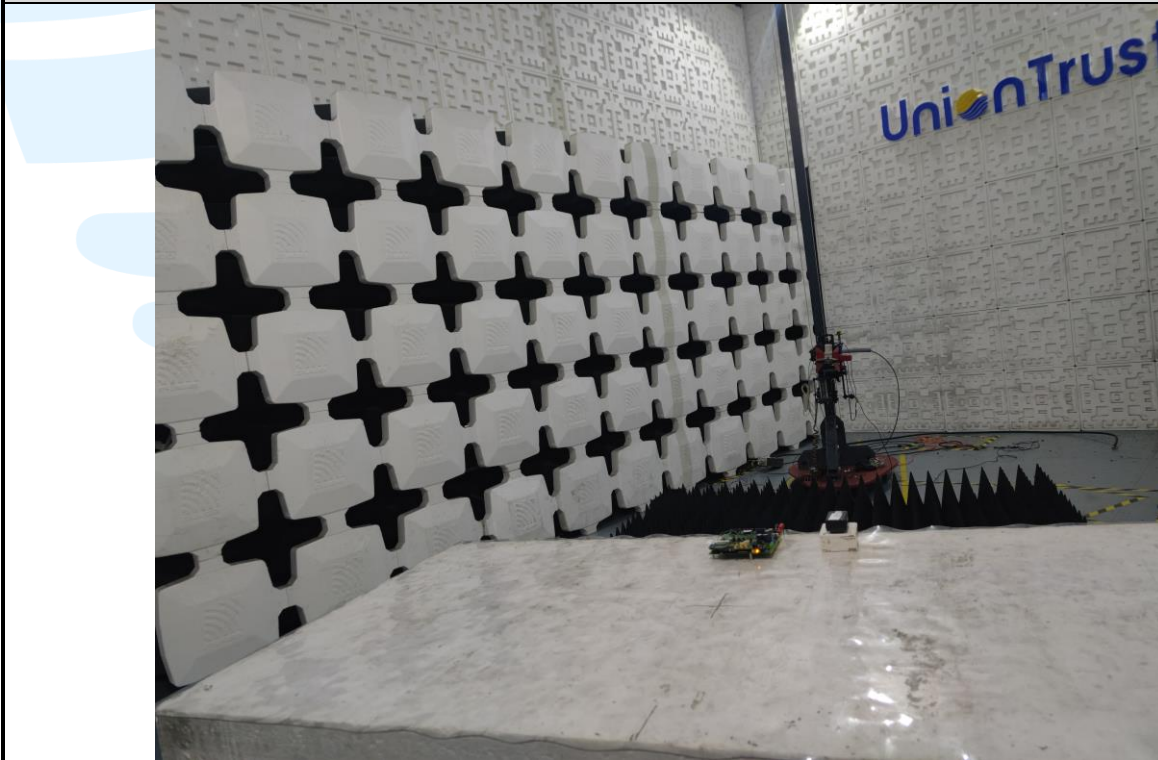
Radiated emission Test Setup-2 (Above 1 GHz)
