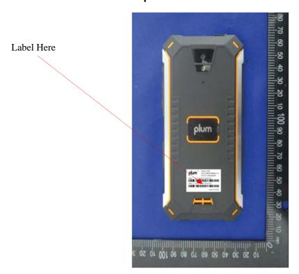
The label shown shall be permanently affixed at a conspicuous location on the device and be readily visible to the user at the time purchase (Labeling requirements per 2.925)
