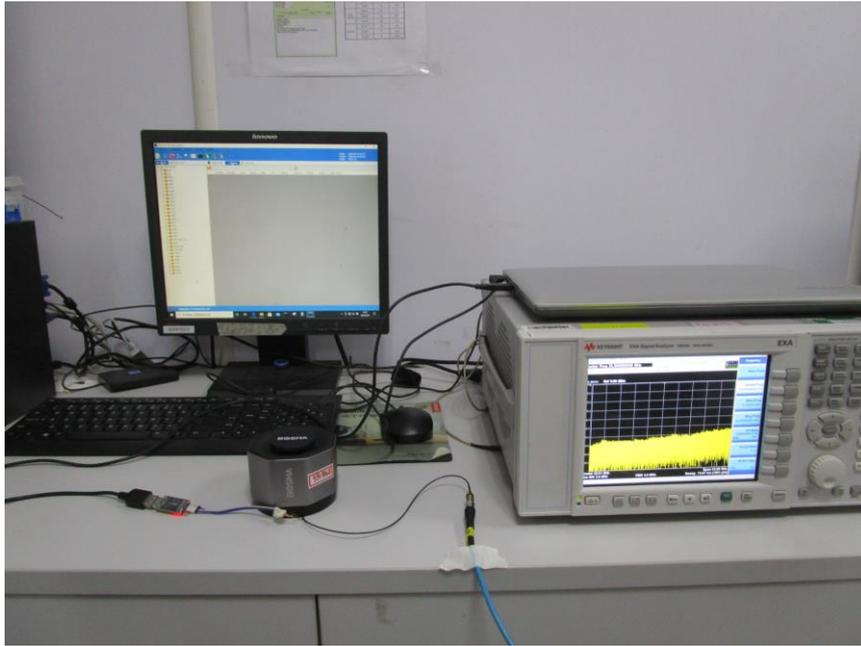
**1.2 Radiated Spurious Emissions & Radiated Emissions which fall in the restricted bands Test Setup**
