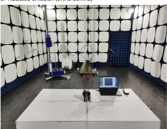
3. Radiated emission (9KHz-30MHz)
