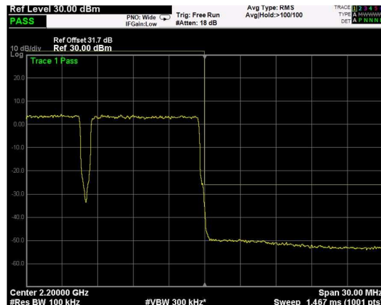
High Band Edge, 2 Carrier, Modulation: 256QAM, BW=10MHz
