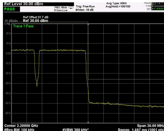
High Band Edge, 2 Carrier, Modulation: 64QAM, BW=10MHz
