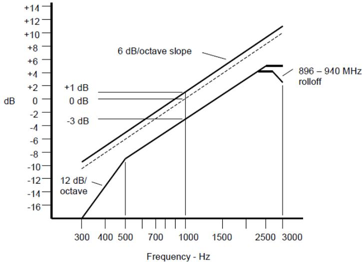
An additional 6 dB per octave attenuation is allowed from 2500 Hz to 3000 Hz in equipment operating in the 25 MHz to 869 MHz range.
