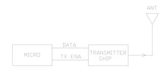
U1 is the Encoder ('Micro') U2 is the single chip transmitter.
