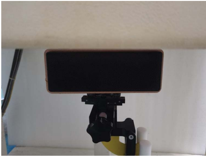
Fig-4.1 Top Side of EUT with 0 cm Gap (Body Mode)
