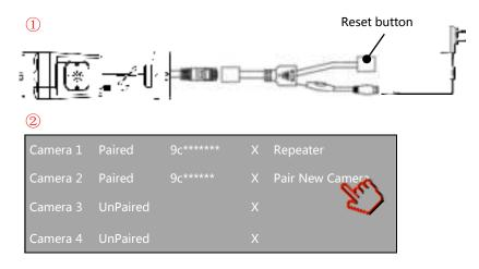
①Power on the cameras and monitor and press reset button
