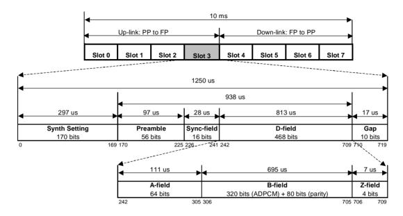
The basic, repeating, frame structure is 10 ms long. It is sub-divided into 8 slots, each  $1250 \mu \text{s}$  long. The active transmission time is  $937.5 \mu \text{s}$ . The first 4 slots form the 'up-link', when the PPs transmit to the FP. The last 4 slots form the 'down-link', when the FP transmits to the PPs.
