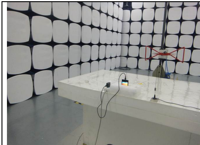
Radiated Spurious Emissions Test Setup Below 1GHz
