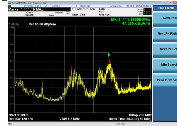
802.11b | Channel 6 | 1 Mbps | 30-200 MHz | Vertical
