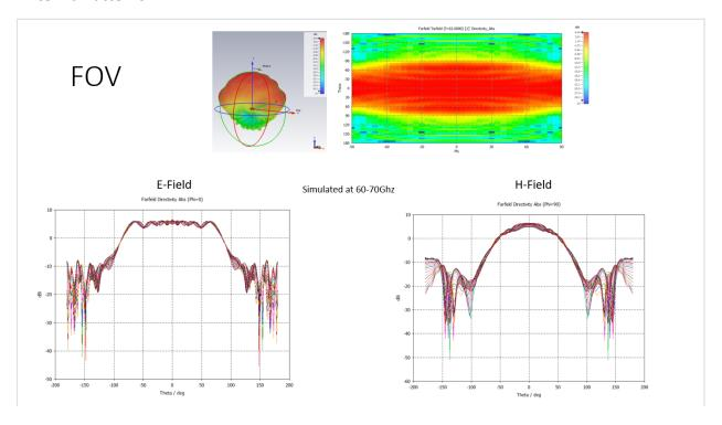
**Test Method and Parameters:** Antenna gain values are determined using FDTD computational analysis. The antenna gain submitted to FCC is based on simulation by a proven and reliable electromagnetic simulation software (CST – one of the industry standards). The simulated performance is in good correlation with the theoretically anticipated value corresponding to a dipole radiating into a half-space (due to a ground plane).
