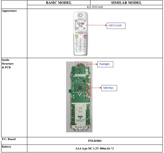
(1) Both models use same portable unit KX-TGUA40 with 2.1 inch LCD.
