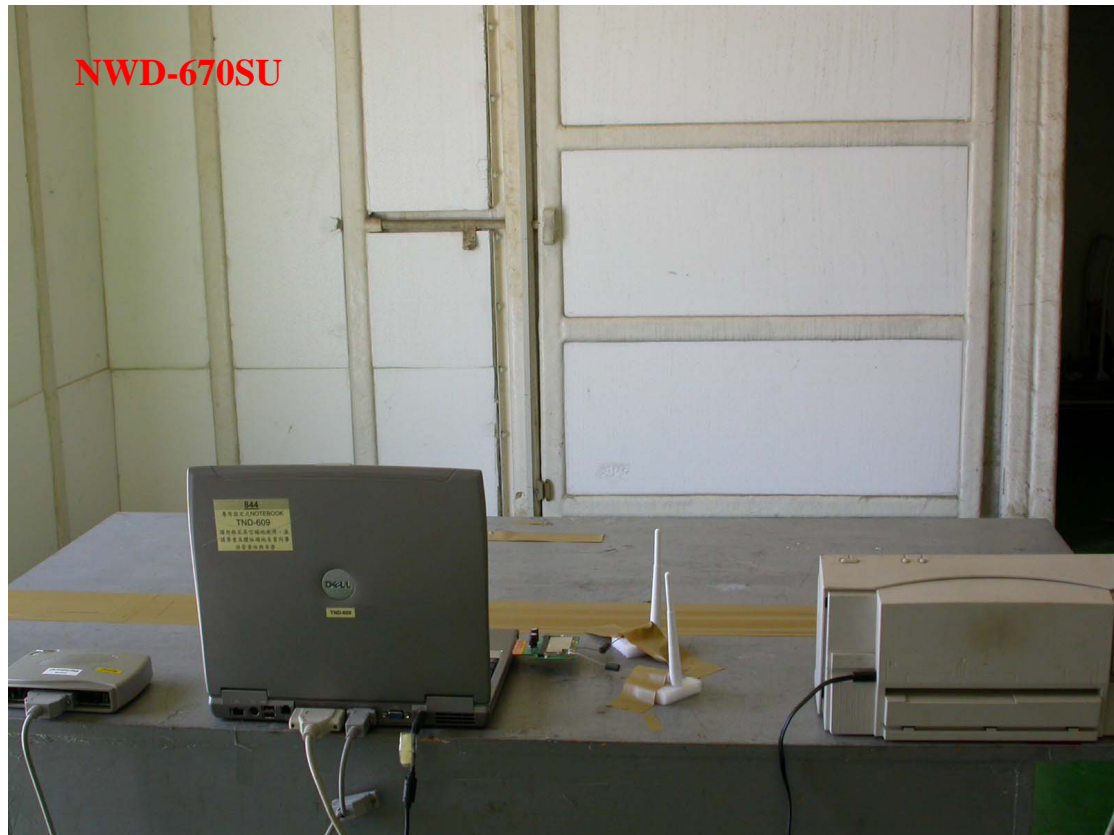
Photo 3: Radiated Emission Test set-up photo
