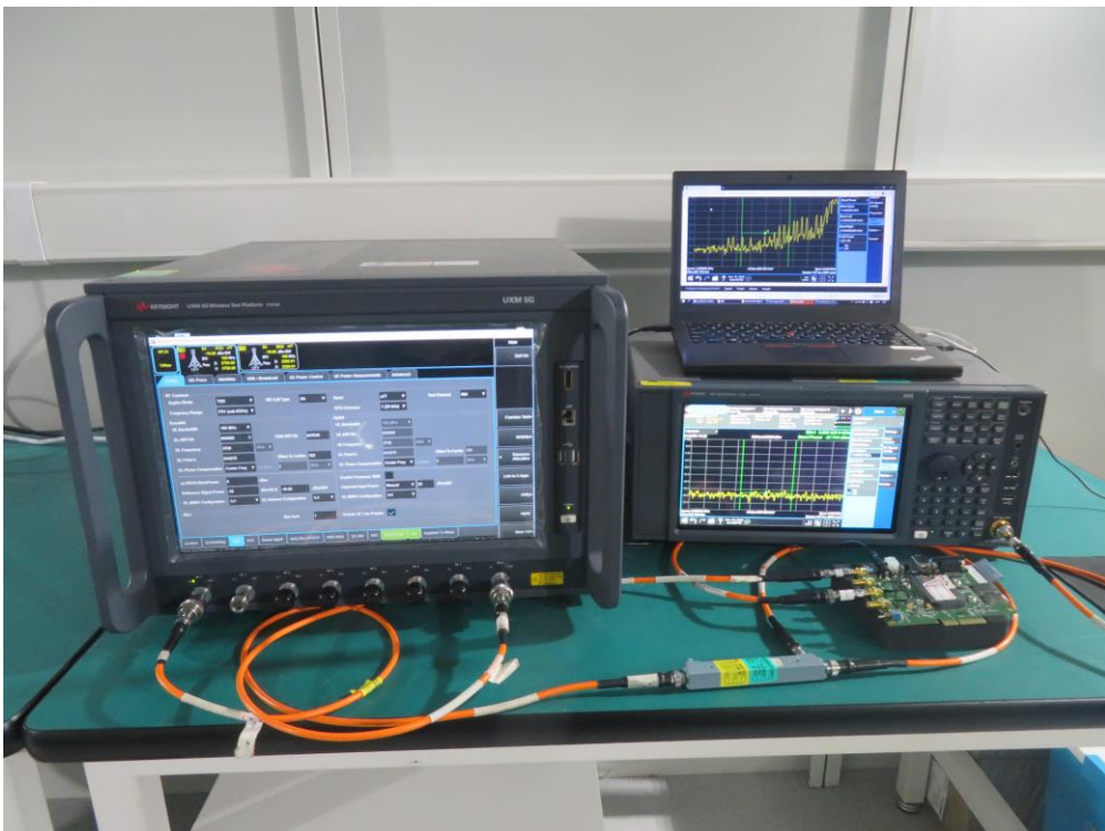
Description: Conducted Measurement Test Setup
