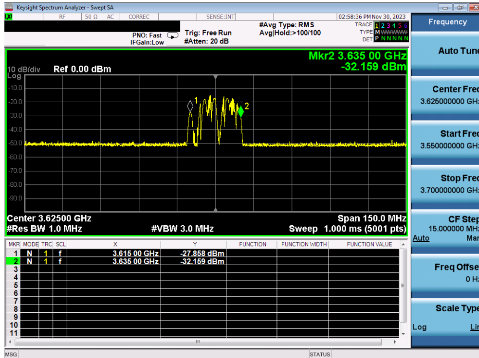
Plot 7. Conducted Measurement – UUT RF transmission range and bandwidths are less or equal to frequency range and bandwidth of compatible BTS-CBSD (WINNF.FT.C.REG.16)
