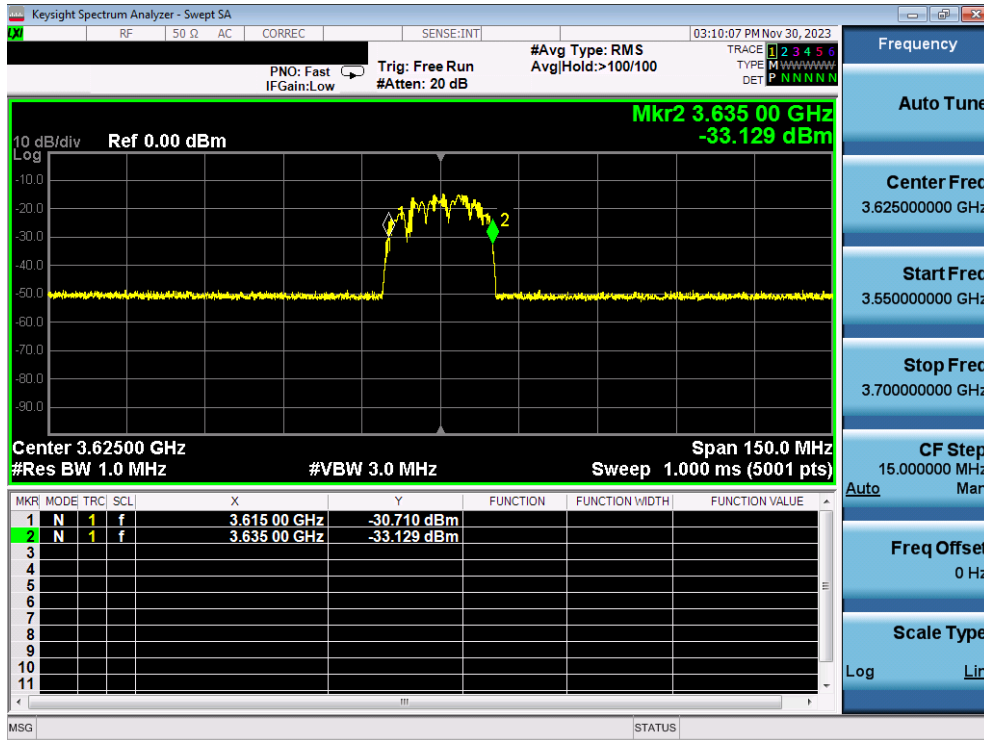
Plot 16. Conducted Measurement – UUT RF transmission range and bandwidths are less or equal to frequency range and bandwidth of compatible BTS-CBSD (WINNF.FT.C.HBT.7)
